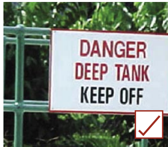
Barricades and warning signs should be placed to prevent fall into uncovered tanks
